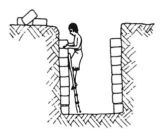
For the direct pit latrine, the slab and water seal pan should be securely fixed to the lining of the pit with cement mortar.
