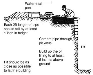
In the case of the mound latrine, first line the sides of the pit and build the lining up to 4ft above ground level.
