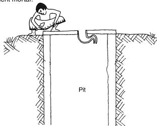
Cover the pit with a reinforced concrete slab. If the pit is large, two slabs may be needed.
